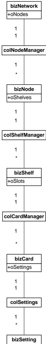
Figure 10. The business object hierarchy for the Network Management System features alternating scalar objects and collections.
