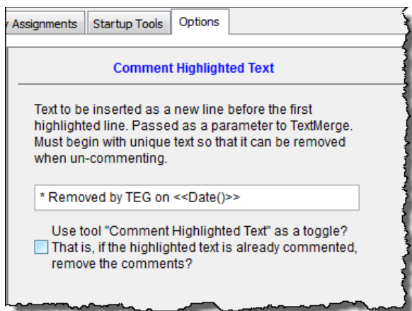
Figure 5. Modifying the header comment on the Options tab changes what the Comment Highlighted Text tool inserts.
