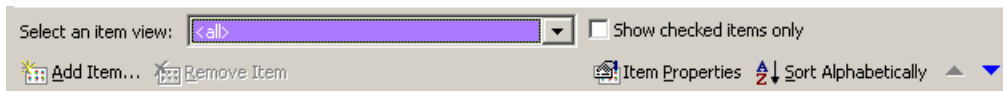
Figure 19. Managing items in the Customize Toolbox dialog. When the item view is set to “<all>,” the button bar lets you work with individual items. The up and down arrows let you rearrange items in the category.
