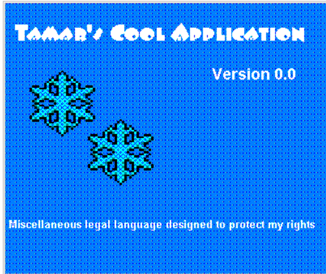
Figure 4 – The new TitleBar property makes it much easier to create splash screens, as well as being useful for ActiveDocs.
